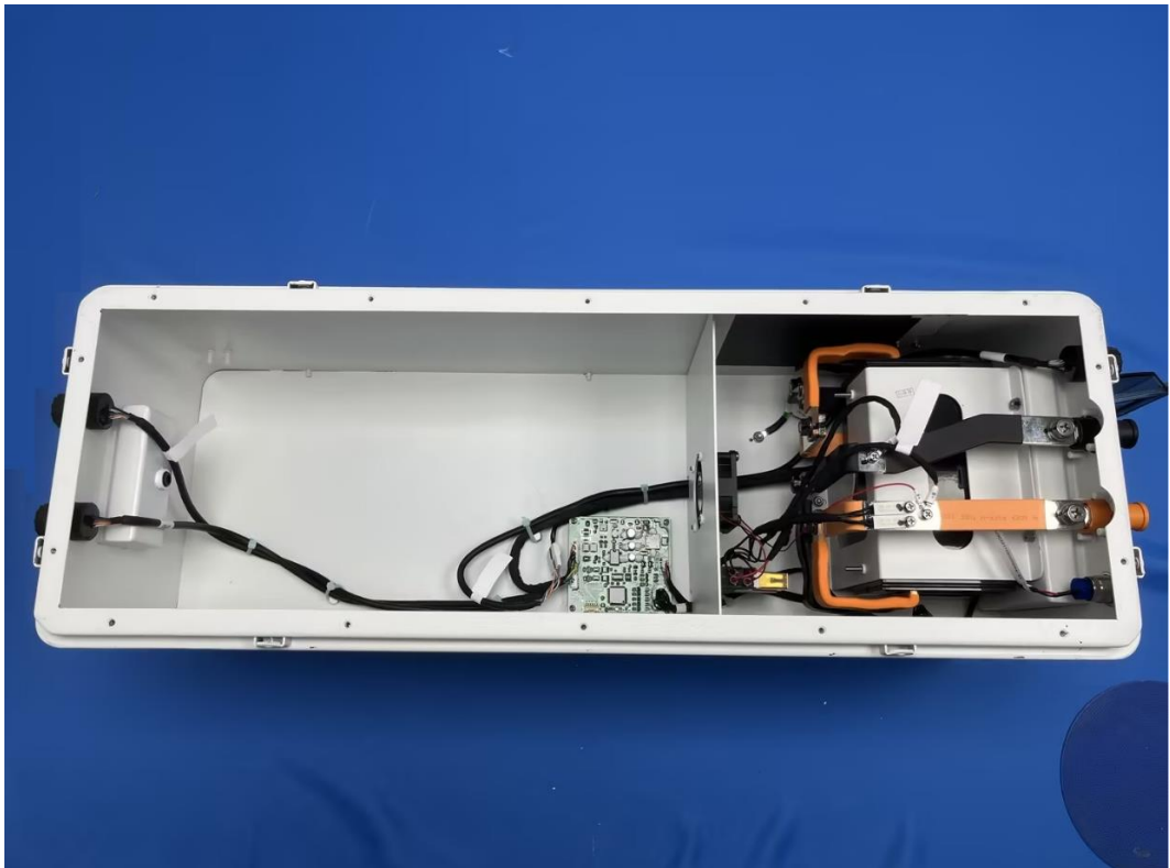
Internal view of PDU (For model: AI-W5.1-B)
